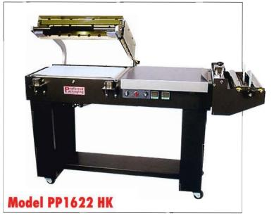
**Hot Knife Seal Head** for PVC or Polyolefin Film — Solid Seal Bar, no wires to replace.
