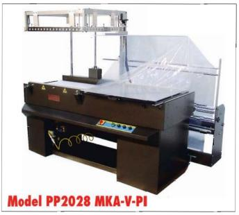
**Air Operated Seal Head**, Push Button Operation. Vertical Seal Head with Powered Film Unwind and Adjustable Inverting Head to Accommodate Tall Packages Up to 18" High.
